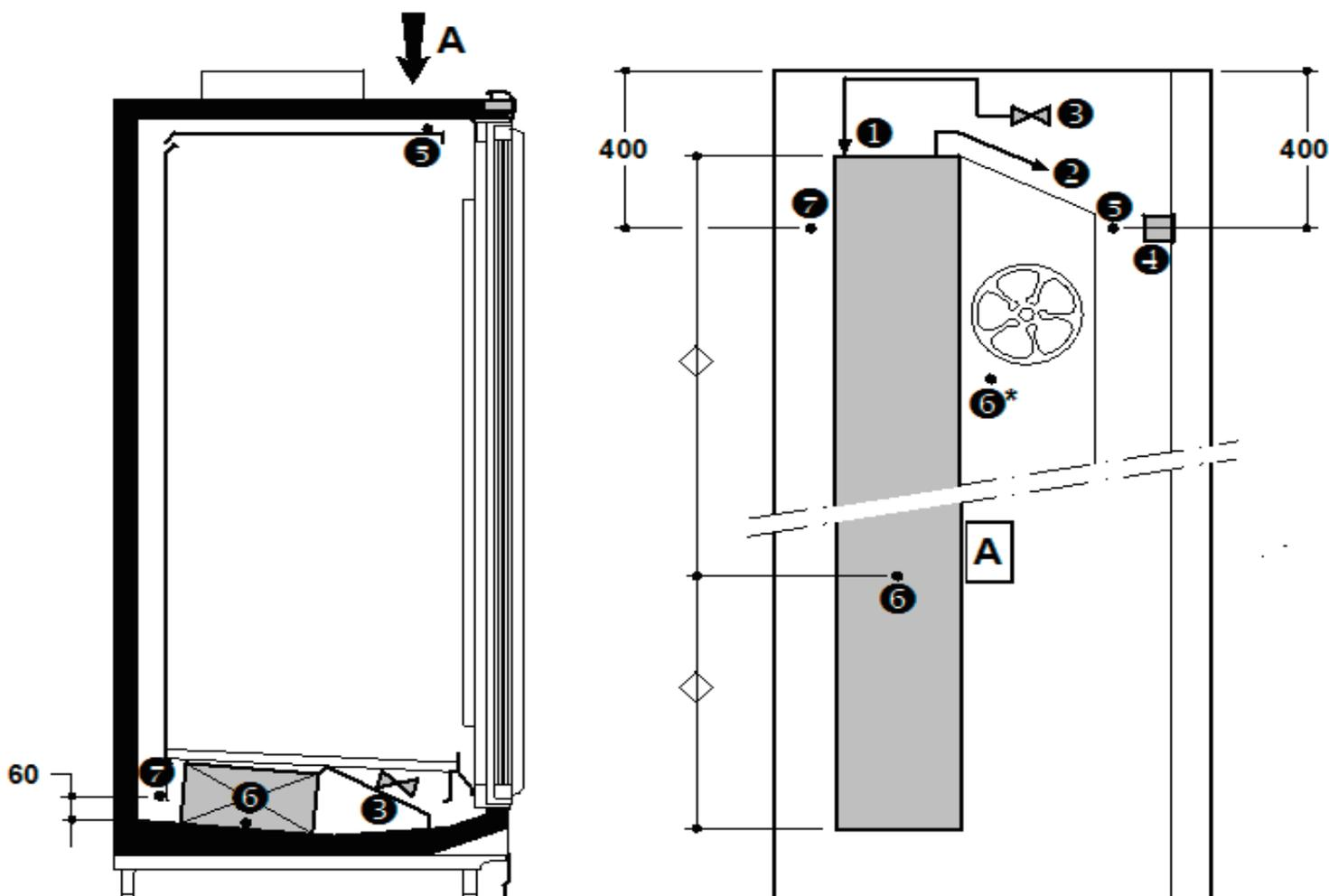
Electrical end defrost probe **6** is located in the middle of evaporator length
